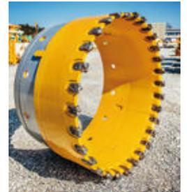
*With increased operational demands and for long drilling tools, use of the long version of the casing shoe is recommended as the most intense strain occurs on the inner surface of the casing shoe in the area of drilling tool action. At this point, the solid-walled construction of the casing shoe ensures a long service life for the entire drill string.*
